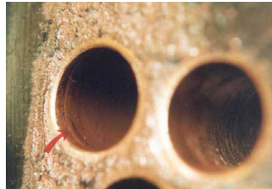
Tube on upper far left with Red arrow has been cleaned and coated with ACE DuraFlo™ Thermal Conductive Epoxy Coating.
